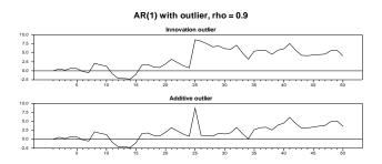
Figure: An innovative (added to the equation) and an additive (added to the process) outlier in the model  $y_i = \beta y_{i-1} + \varepsilon_i$  i.i.d.  $(0, \sigma^2)$
